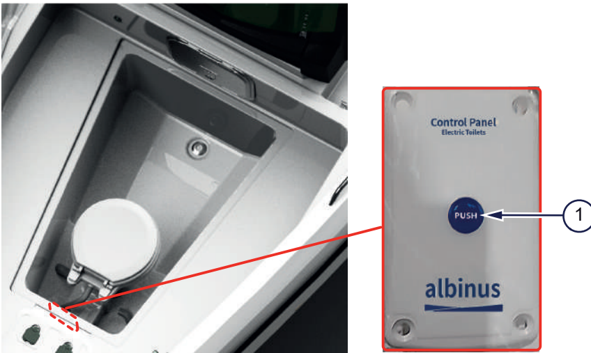
Figure 4.8 - Toilet compartment control panel
