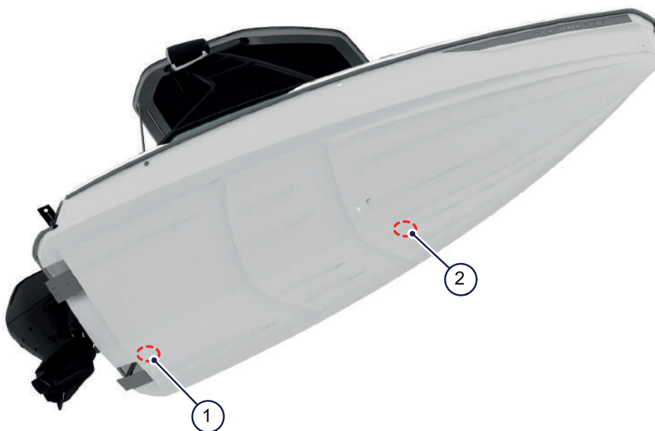
Figure 5.4 - Automatic bilge pumps
