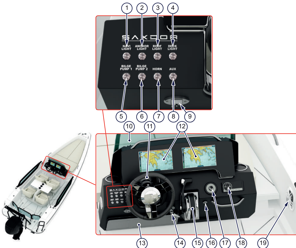
Figure 4.7 - Helm station controls
