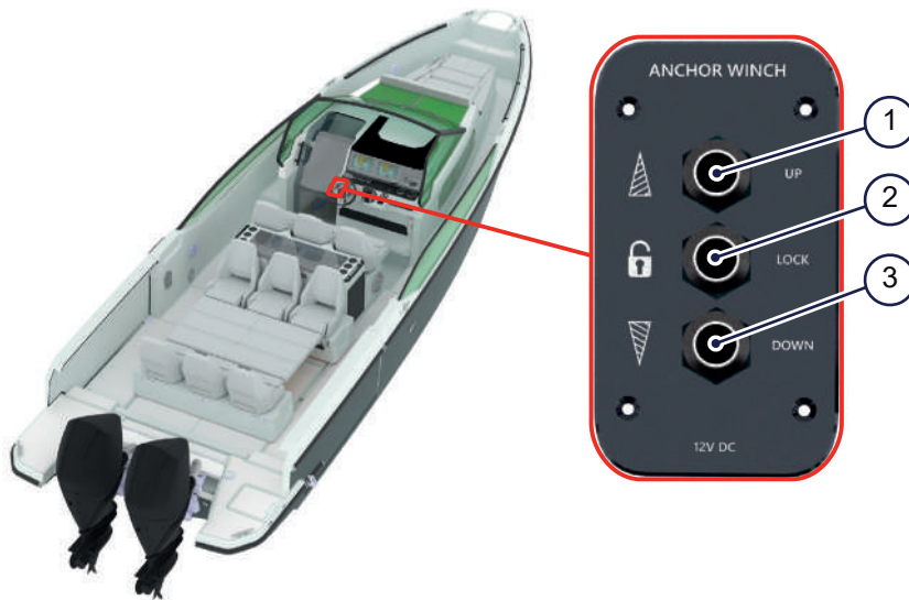
Figure 4.5 - Anchor winch control panel
